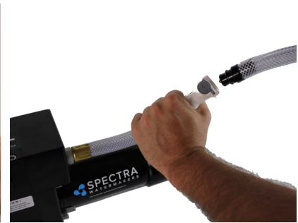
Connecting brine discharge service hose
