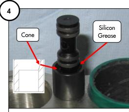
Place the assembly tool over the borehole with the cone-shaped taper on top.
