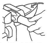
Identify Over All Length (OAL) of hose assembly and the Cut Off Allowance (COA) length of fitting(s) on hose ends by use of the fitting data table. Properly measure, mark and cut hose to desired length using fine tooth hacksaw or a cutoff machine. Place socket in vice and screw in hose counter-clockwise until hose bottoms. Back hose out 1/2 turn.
