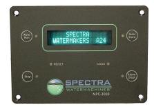
The system will go into a start mode and the Spectra-Pearson Pump will start shortly after. The system should prime within 60-90 seconds. Check the strainer and the brine discharge for water flow. There should be no bubbles anywhere in the intake hoses and the Spectra-Pearson Pump should sound smooth after priming. If it continues to sound rough, find the reason before continuing! Inspect the system for leaks.
