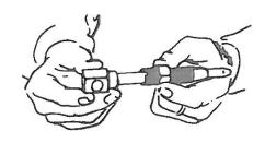
2. When assembling male pipe ends, slide nipple onto mandrel.
