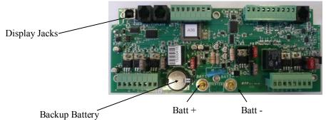
Connect DC power to the Batt + and Batt - posts on the MPC board, pictured above. DC power feeds should be sized for 10 Amp maximum supply and be uninterruptible to insure proper operation of the auto store feature. Avoid house breaker panels that could be easily tripped. Connect the DC power cables directly to the battery positive and negative posts on the MPC board.
