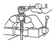
When assembling swivel ends, screw threaded mandrel all the way into interior threads of swivel and wrench tight.
