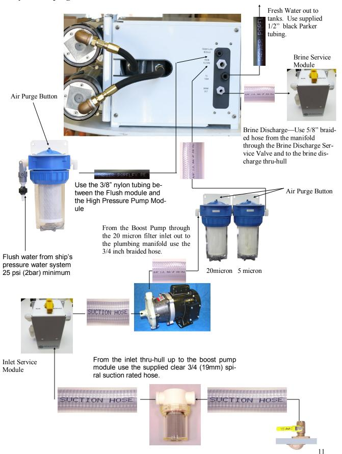
**Note!** When plumbing the Farallon High Pressure Module route the feed water so that the top and side covers may be opened without removing the hoses or tubing.
