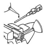
4. Oil nipple threads and inside of hose with silicone oil or diluted soapy water. DO NOT OIL HOSE COVER
