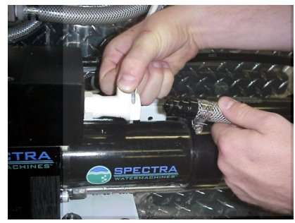
Connecting brine discharge service hose
