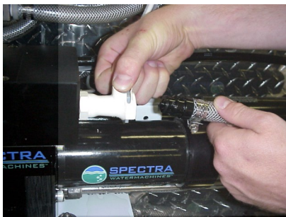
Connecting brine discharge service hose
