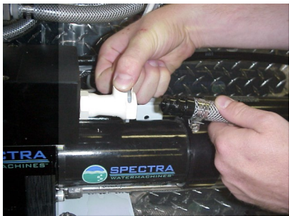
Connecting brine discharge service hose
