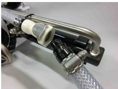
Connecting brine discharge service hose
