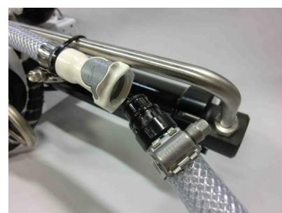
Connecting brine discharge service hose
