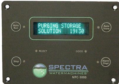
*If the system continually alarms 'Service Prefilter' at the beginning of the purge sequence, then air may be trapped in the prefilter housings. Use the 'Air Purge Button' on top of the filter housings to evacuate the trapped air, and try again.*
